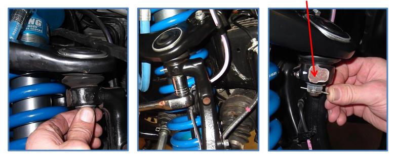
11. Reconnect tie rod end to the steering knuckle and tighten nut to factory specs. Be sure to insert the cotter pin through the castle nut and bend the ends as shown.
